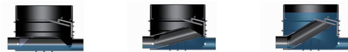
The first figure shows the WaBack in normal operation, the WaBack is always open. The mid figure shows the event when a reversed flow occurs, the float begins to rise. The final picture shows the pipe completely sealed against the sealing plate.
