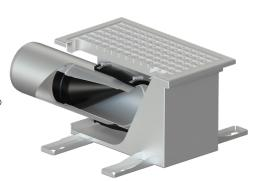
When back pressure occurs from the drainage system and water flows back towards the floor drain, the WaStop Inline check valve prevents water from rising out of the well and further into the property through the door. This ensures that the property remains dry and protected from flooding.
