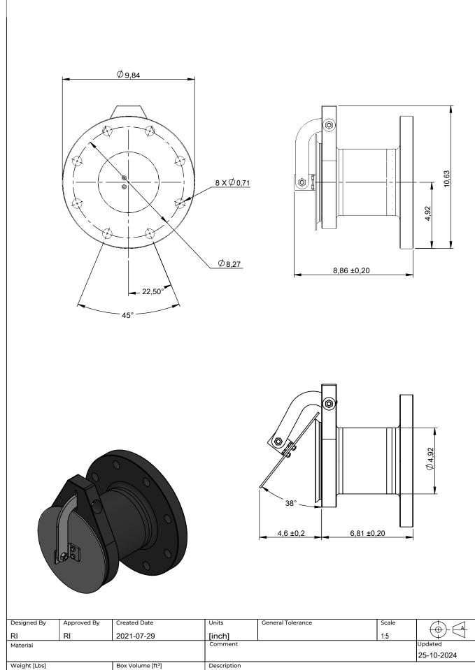
WaFlap Flap valve KVD NPS/OD 5" AISI 316
