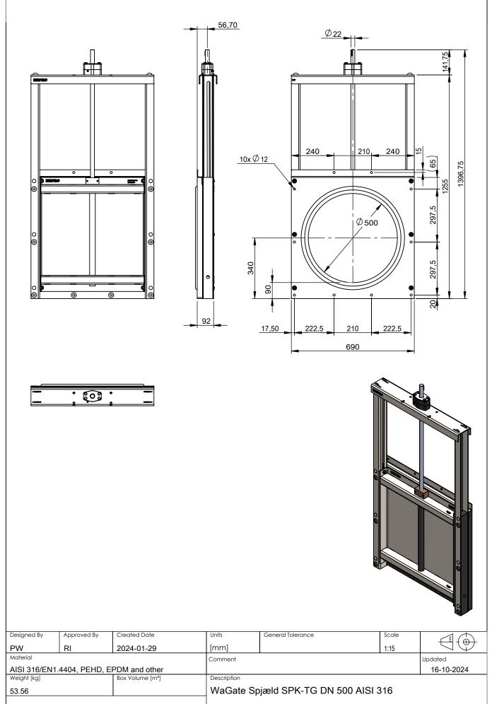
WaGate Sluice gate SPK-TG DN 500 AISI 316
